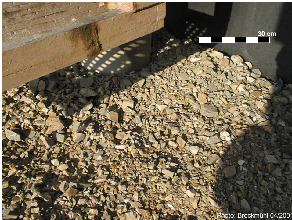
Figure 13 Mud rotary drill cuttings of WW39992 show breccias with ferrous oxide coatings within the dolomite (Hüttenberg formation).
